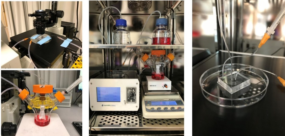
Laboratory set-up of microfluidic sorting and purification of cells during red blood cell culture and manufacturing [Credit: SMART]
